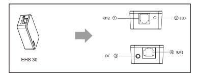
Port ①: RJ-12 Port for IP Phone EXT/EHS or Expansion Moduleusing the RJ12 cord.
